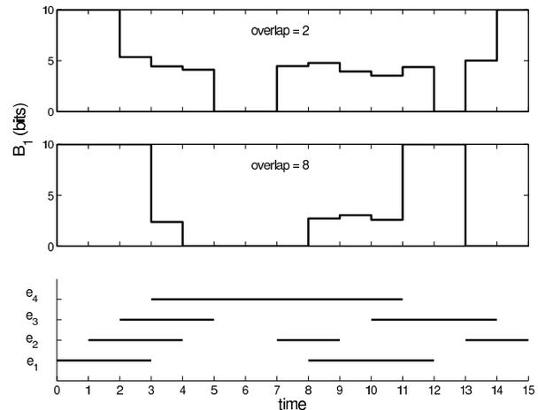
**Fig. 3.** Dynamic bit allocation in a two-subspace system. The top two plots depict  $B_1$ , the bit allocation to  $W_1$  resulting from maximizing  $\gamma$ . At any time each of four events may be present. For the top plot, the two feature subspaces share two common dimensions, whereas for the middle plot they share eight dimensions. In the high-overlap case, bits are more often allocated to a single subspace. The bottom plot indicates the events present at each time step.
