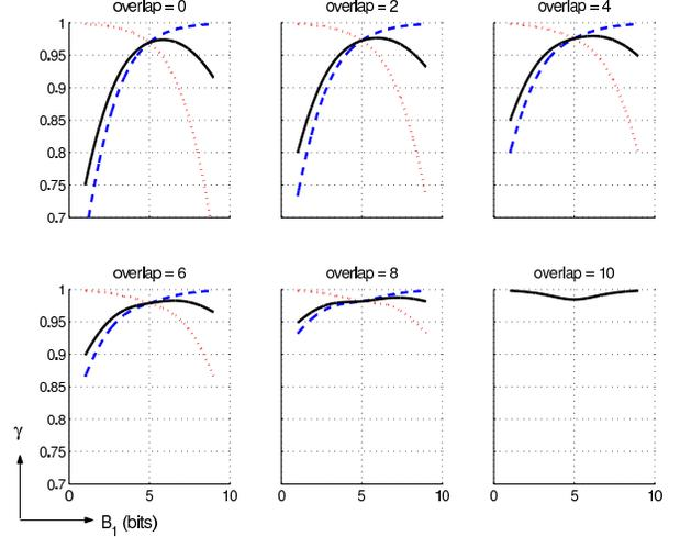
**Fig. 2.** Information transfer vs. bit allocation to one subspace for a two-feature system. Shown are the information transfer ratios for two events  $e_1$  (dashed) and  $e_2$  (dotted) with priorities  $\alpha_1 = 3/4$  and  $\alpha_2 = 1/4$ . The solid curve is the priority-weighted sum  $\gamma$ . With increasing overlap between features, allocating more bits to  $W_1$  maximizes  $\gamma$ .
